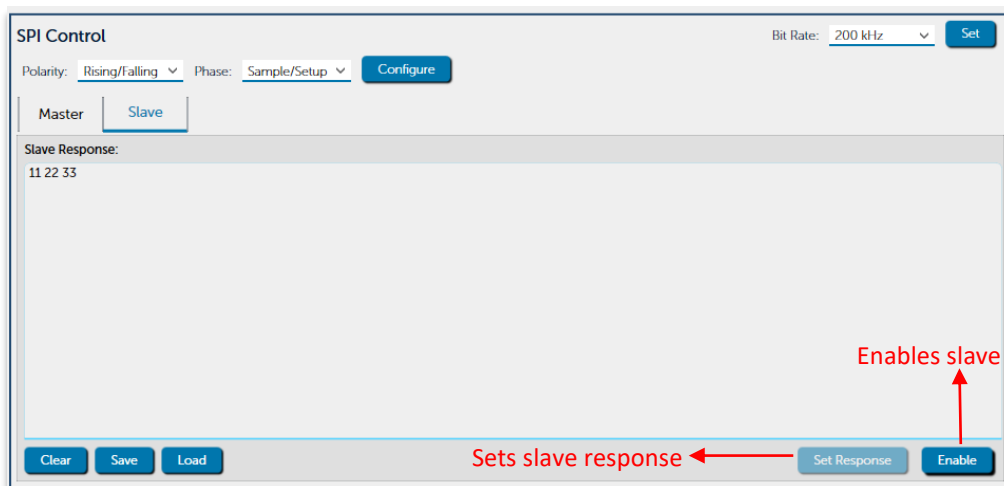
Figure 27: SPI slave control panel
